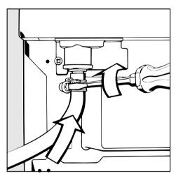
■ Detach the hose clip from the drain outlet at the back of the machine and remove the rubber plug.
